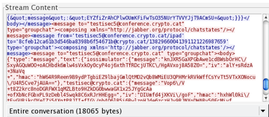
Figure 7: Cleartext XMPP stream captured by Wireshark after performing the StartTLS stripping attack
